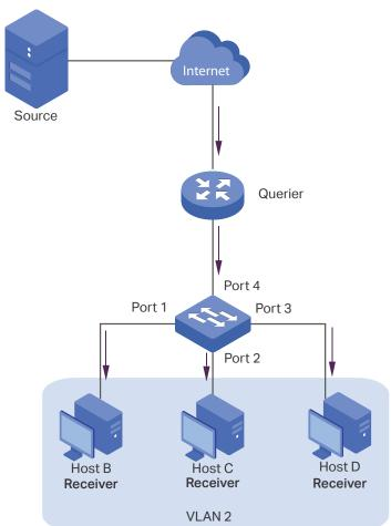
Figure 5-1 Network Topology for Basic IGMP Snooping
