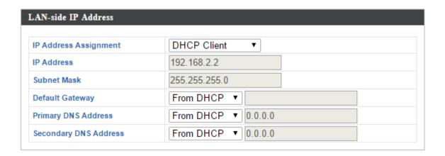
2. Enter the IP address settings you wish to use for your access point. You can use a dynamic (DHCP) or static IP address, depending on your network environment. Click "Apply" to save the changes and wait a few moments for the access point to reload.
