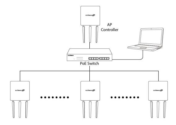
5. Open a web browser and enter the AP Controller's IP address in the address field. The default IP address is 192.168.2.2
