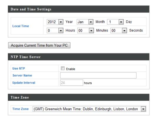
**9.** Set the correct time and time zone for your access point using the drop down menus. The access point also supports NTP (Network Time Protocol) so alternatively you can enter the host name or IP address of a time server. Click "Apply" when you are finished.
