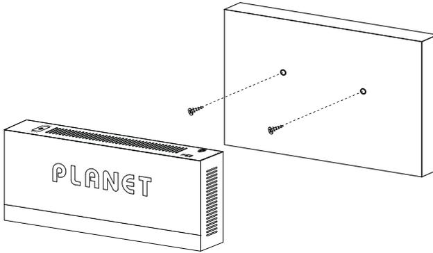
**Figure 3-3:** PoE Ethernet Switch Wall Mount Installation
