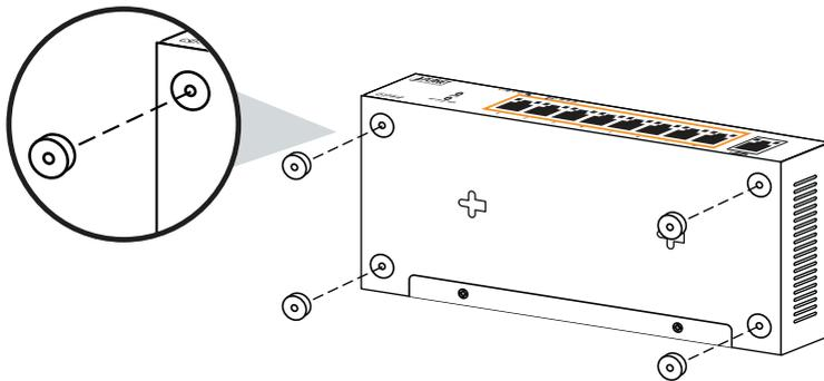
**Figure 3-2:** Installation of PoE Ethernet Switch Magnets
