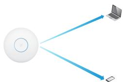
MU-MIMO with 3x3 and 1x1 clients: The UniFi AC HD AP communicates with one 3x3 client and one 1x1 client at a time.
